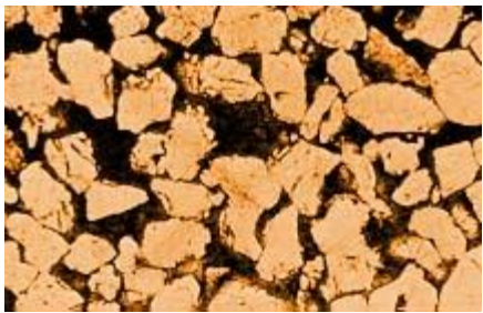
When reservoir rock is magnified, the tiny pores that contain trapped oil droplets can be seen.
