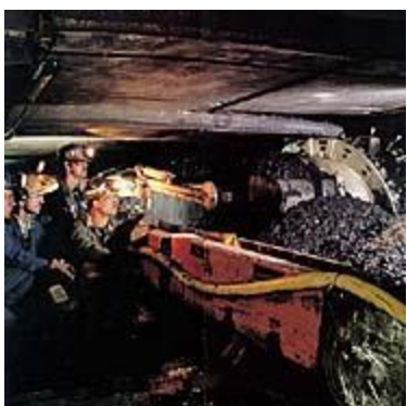
One type of mining, called "longwall mining", uses a rotating blade to shear coal away from the underground seam.
