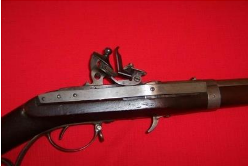
Original Model 1819 Halls flintlock breechloading rifle, breechblock dated 1838, .54 caliber. First machine of any kind made with TOTALLY INTERCHANGABLE PARTS , This was part of the beginning of what was called the "American Method of Manufacture", where less skilled workers could operate machinery to build gun parts, then assemble the whole gun. People from all over the world came to Harpers Ferry to see this wonder of modern manufacture. As of April 2013 the Model 1819 Hall Rifle has been adopted by the WV Legislature as the Official State Firearm of the great State of West Virginia.
