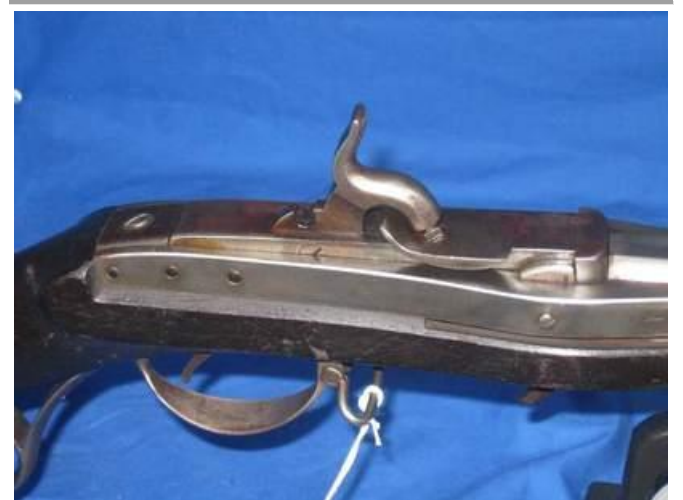
Model 1819 Halls breechloading originally flintlock rifle, converted to percussion. Breechblock dated 1831, .54 caliber. Not only did John Hall invent and patent his breechloading rifle in 1811, he went on to patent several machines used in the manufacture of his interchangeable parts system. These patent records were lost in a fire at the US Patent office in Washington, DC.
