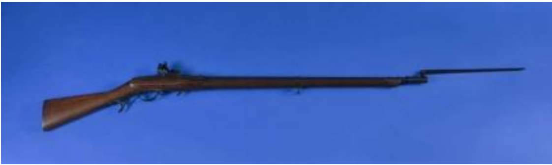
Original Hall Model 1819 flintlock breechloading rifle, with stock shattered due to blown breech. This was a flaw with the Hall's rifles; when the breechblock was loaded and seated, gunpowder or other elements could become lodged in the seat, causing the gun to blow gas out the sides of the breechblock chamber upon discharge. Breechblock dated 1834.
