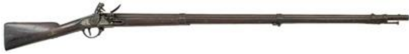
Original Harpers Ferry Model 1795 flintlock musket, .69 caliber, lockplate 1816. These guns were the first model produced by the Harpers Ferry & Springfield National Armories, patterned after the French Charleville musket.
